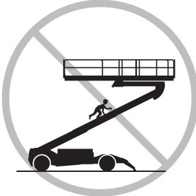
DO NOT EXIT PLATFORM WHEN ELEVATED
