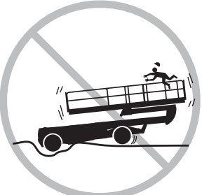
DO NOT DRIVE ON IRREGULAR OR UNSTABLE SURFACE
